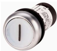
**Illuminated pushbutton actuator, Flat, momentary, 1 N/O, Screw connection, LED white, White, inscribed, 24 V AC/DC, Bezel: titanium**
